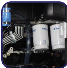
Fuel particle separator filter
