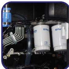
Fuel particle separator filter
