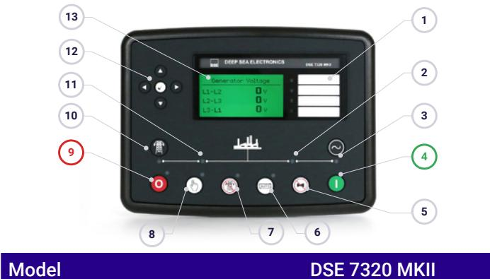
DSE 7320 MKII DEEP SEA control card with mains grid monitor. The genset will automatically start up when detecting a fault in the electric power network and it will turn off automatically as well, when the electrical supply is re-established. It can also work in manual mode and by signal. It allows you to monitor a wide range of generator parameters and display information alerts, status and alarms.
