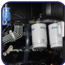
Fuel particle separator filter
