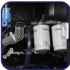
Fuel particle separator filter
