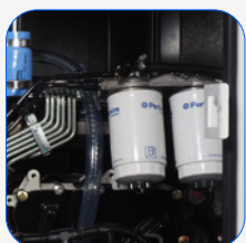
Fuel particle separator filter
